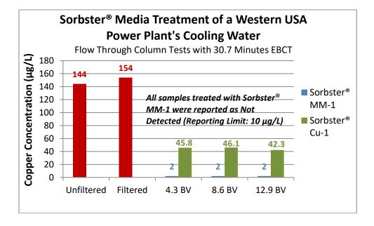
Removal of copper is shown for both Sorbster<sup>®</sup> MM-1 and Sorbster<sup>®</sup> Cu-1 media types. Sorbster<sup>®</sup> MM-1 achieved a >93% removal rate and Cu-1 a 72% removal rate. Sorbster<sup>®</sup> MM-1 demonstrated sustained copper removal to single digit ppb levels and met the plant target of <0.01 mg/L.
