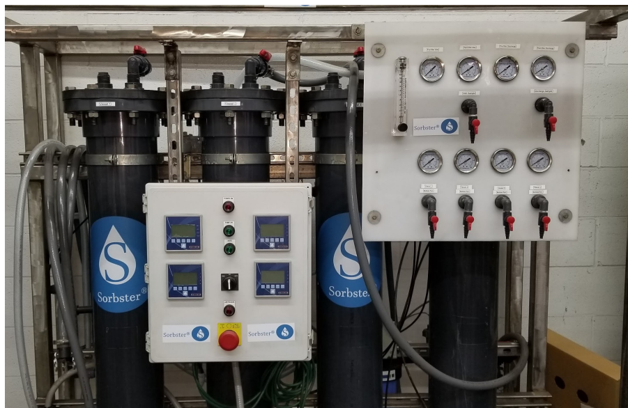
Image - The Sorbster® Media Treatment Unit consisting of four vessels plumbed for series water flow. This unit is equipped with inlet and outlet pH measurement, inlet water conductivity, a pump, flow controllers, flow totalizers and pressure drop
